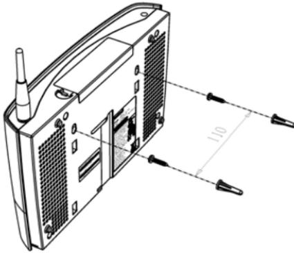
Insert and secure two screws in the wall at a distance of 110 mm. Leave a space of approximately 3 mm between the surface and the bottom of the screw heads. Slip the Ericsson W25 slots over the screw heads and pull down until the unit is seated securely.
