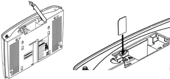
**NOTE!** *The Ericsson W25 must be disconnected from the power mains or an optionally installed battery when inserting or removing the SIM card.*
